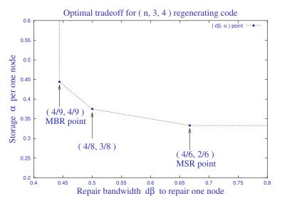
Optimal tradeoff curve between strage  $\alpha$  and repair bandwidth  $d\beta$  for (k, d) = (3, 4) and B = 1.
